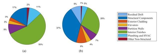
Figure 4. Contribution of different building components to the overall loss at the Design Earthquake: (a) Site Class B and (b) Site Class D.
