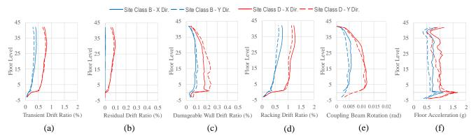
Figure 3. Mean demands from nonlinear response history analysis at the Design Earthquake: (a) transient drift, (b) residual drift, (c) damageable wall drift, (d) racking drift, (e) coupling beam rotation, (f) floor acceleration.
