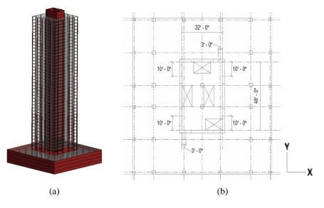
Figure 1. Archetype Reinforced Concrete Shear Wall building: (a) isometric view and (b) plan view. Adapted from [9]. Table 2. Dynamic vibration periods of the Reinforced Concrete Shear Wall building. Adapted from [8].
