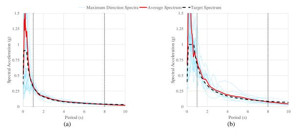
Figure 2. Design Earthquake target spectrum superimposed with the suite average and individual ground motions spectra: (a) Site Class B and (b) Site Class D.
