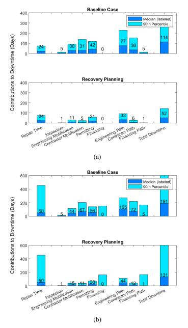
Figure 5. Downtime de-aggregation at the Design Earthquake with and without recovery planning: (a) Site Class B and (b) Site Class D.
